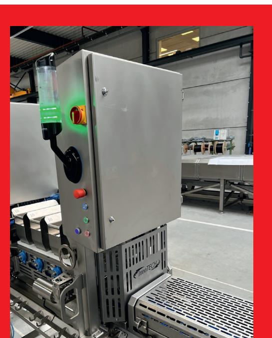
The LED signal towers clearly and reliably signal the current status of the production line in the common traffic light colors red, yellow and green
