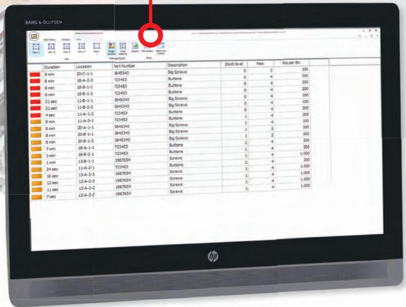
The digital Kanban board (material requirements list) indicates the locations which require replenishment.
